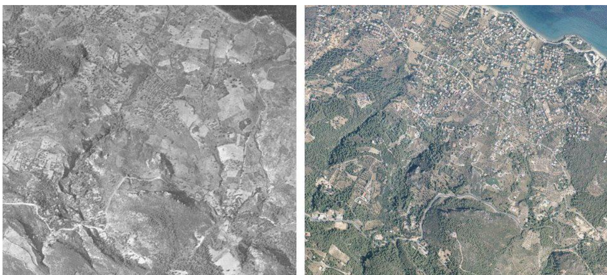
Figure 1: Data sets: aerial photograph captured in 1945 (left), orthoimage made from aerial images collected in 2008 (right).
